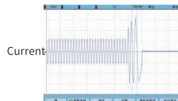
Magnetic flux braking current wave in the SVPWM mode for asynchronous motors Frequency: 50Hz Rated load: 100%
