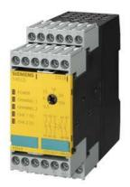
SIRIUS safety relay with relay enabling circuits (EC) 24 V DC, 45 mm overall width Screw terminal EC instantaneous: 2 NO EC delayed: 2NO, 0.05...3 s SC: 1NC monitored start Basic device Maximum achieved SIL: 3/2, PL: e/d
