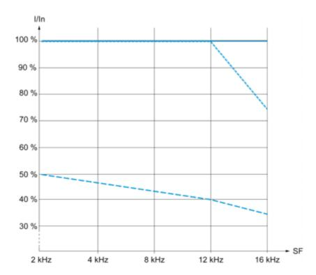
40 °C (104 °F) - Mounting type A, B and C 50 °C (122 °F) - Mounting type C 60 °C (122 °F) - Mounting type C
