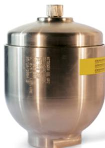
Body in S.S.316, composed by two parts assembled together by means of a special hosing that, under dynamic pressures, tends to close itself. Various diaphragm materials available, for wide chemical compatibility. Built accordingly to the ASME VIII° Div. 1
