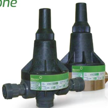
Back pressure valve is installed in line on the delivery pipe of the pump in order to counteract the existing pressure in the suction in order to avoid the siphoning. Use of this valve allows the flow to be regulated in cases where the discharge pressure is low or non-existent.
