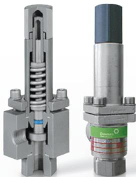
Safety valve is installed on pump delivery pipe and it is jointed to the bypass pipe as a safety device, so it opens (discharges) when the limit value is reached in order to protect the system and pump against pressure overloads.
